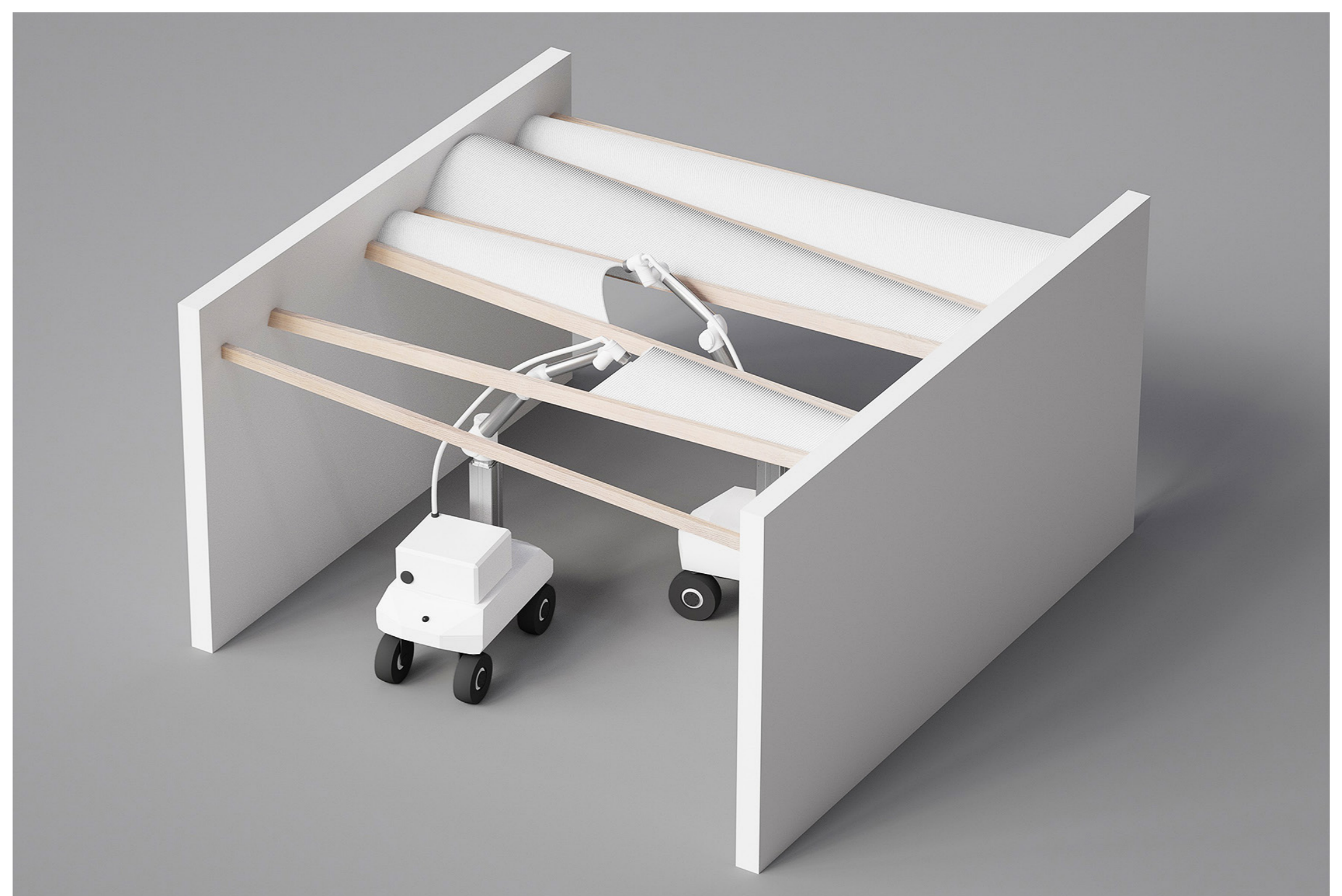
Figure 6.2: Outlook of a potential future fabrication method with multiple mobile robots - Top view
