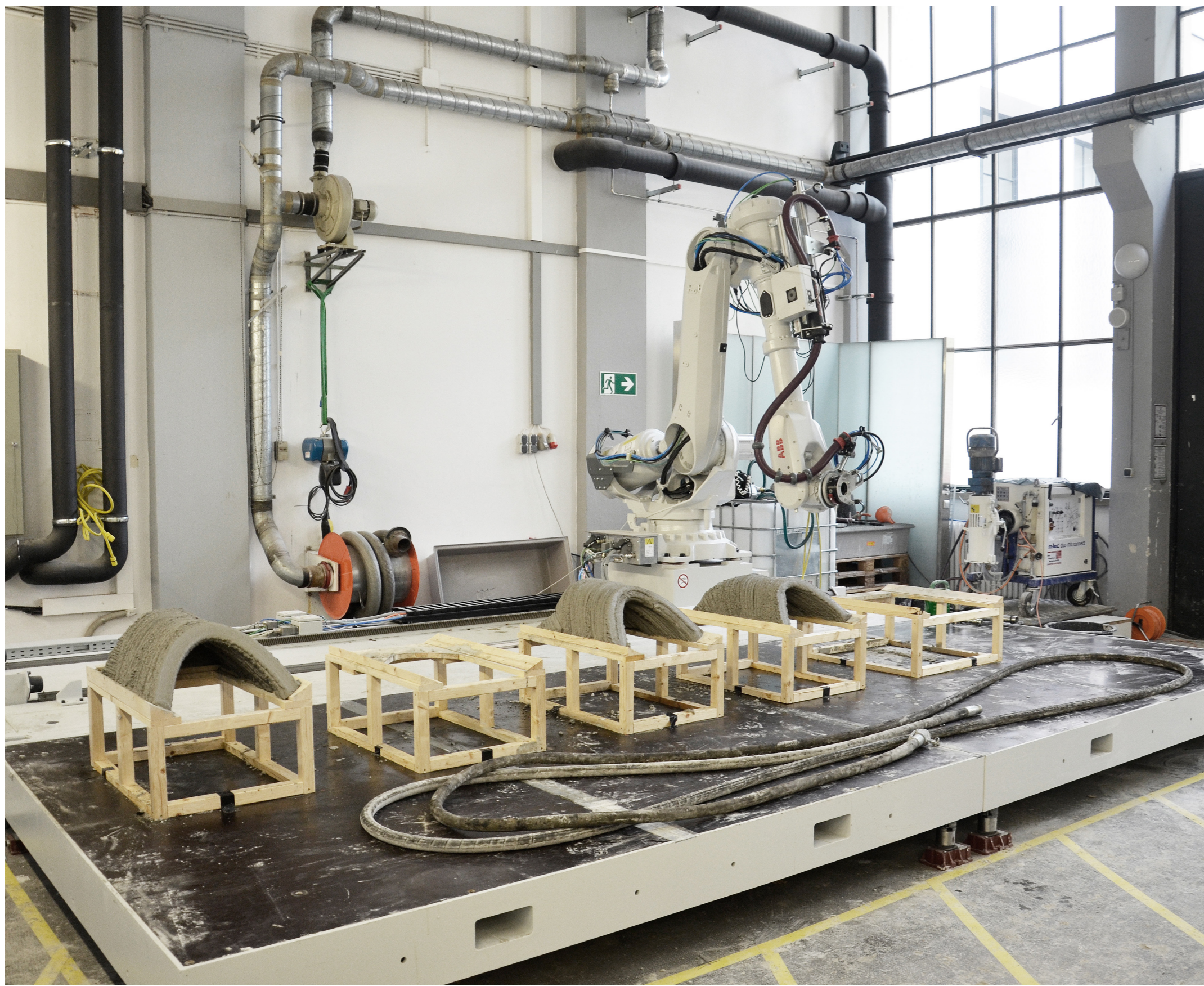
Figure 3.1: Robotic fabrication setup
