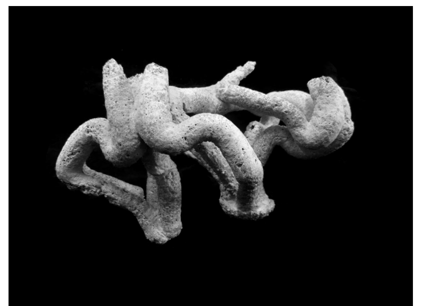
Internal skeleton by I3DCP (cast in lime suspension), block 3
