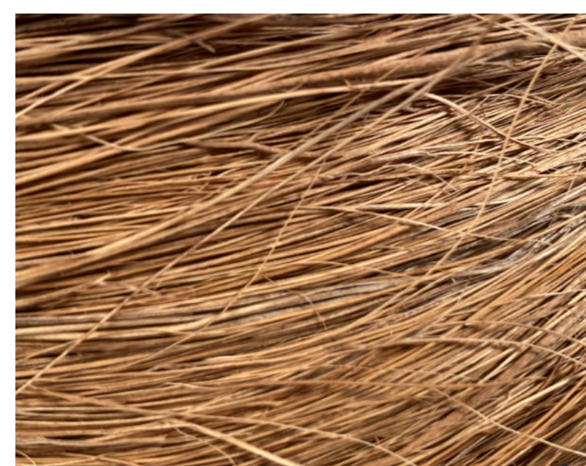
Coir fibre (diameter 0.1-0.5 mm)
