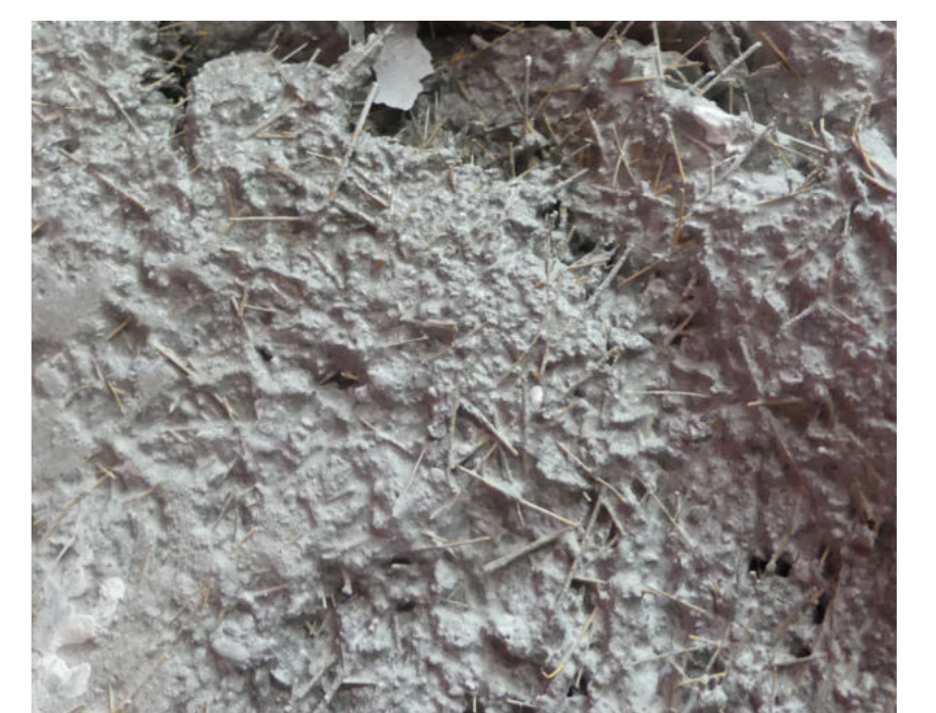
Coir fibre in "muscle" of insulation block)
